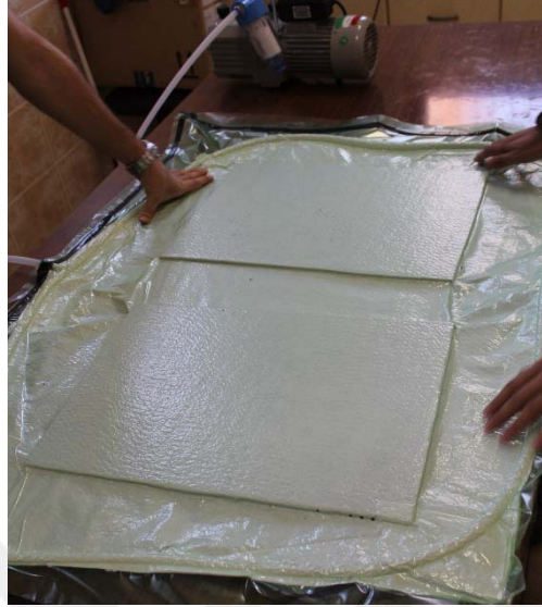
Figure 3.13. Application of vacuum
