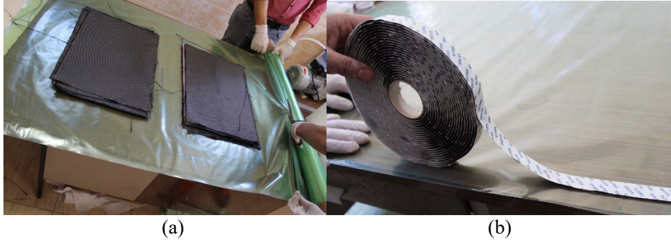
Figure 3.5. Preparing of vacuum bag
