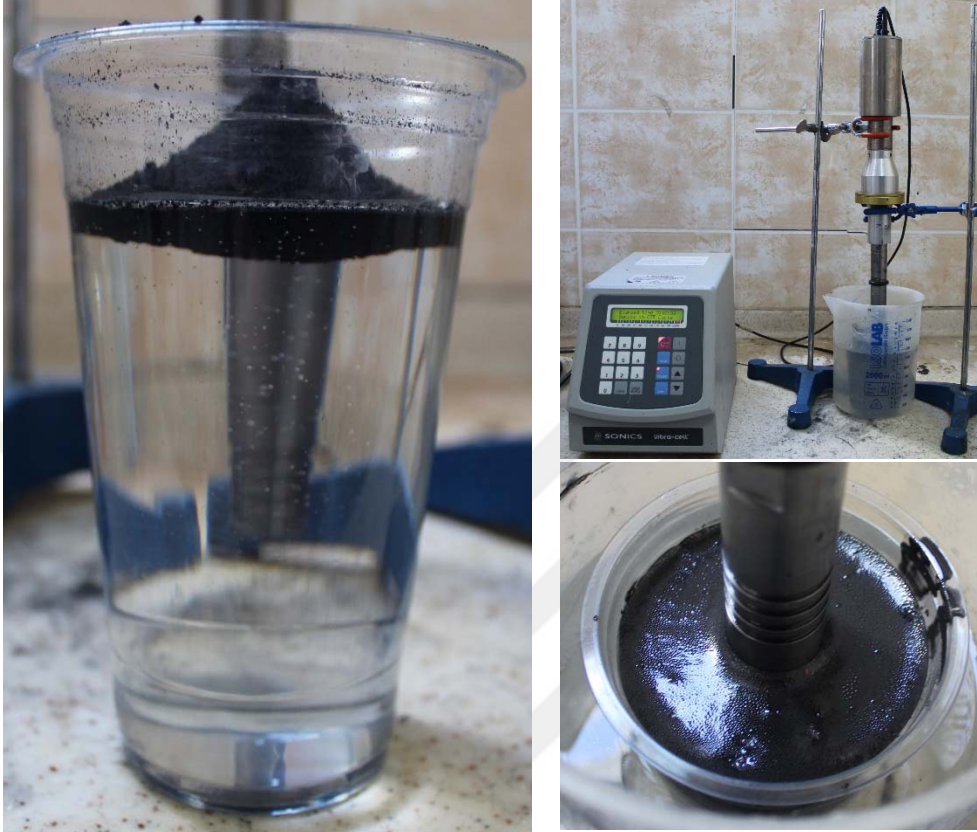
Figure 3.7. Sonication processes of additives
