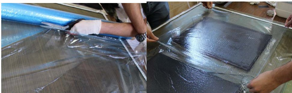
Figure 3.9. Cutting and application of perforated film
