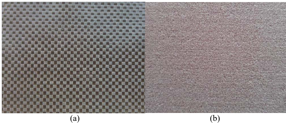
Figure 3.1. Sandwich structure components: (a) woven carbon fiber fabric; (b) closed cell PVC foam
