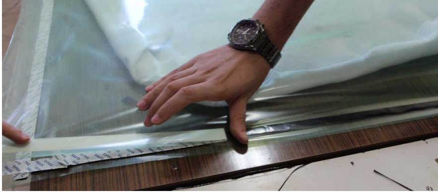
Figure 3.12. Closing the vacuum bag
