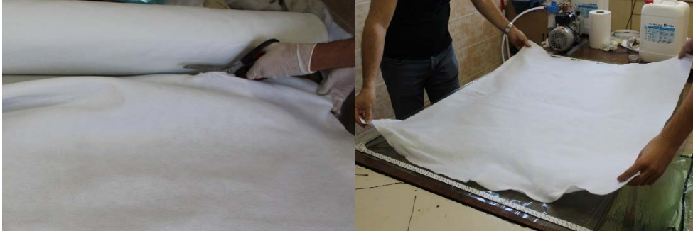
Figure 3.10. Cutting and application of breather
