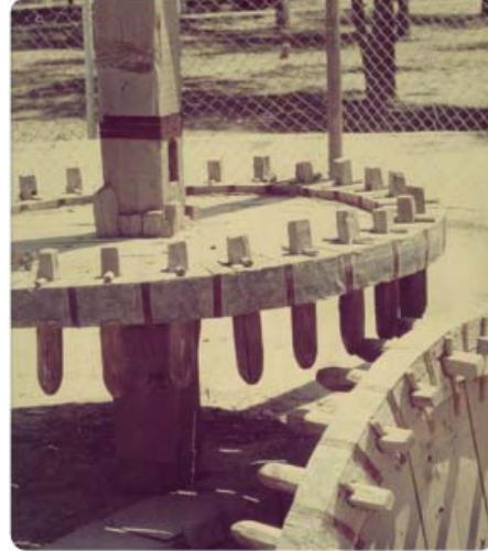
Figure 1.1. Primitive gears made of wood (K.Gopinath & M.M.Mayuram, 2009)
