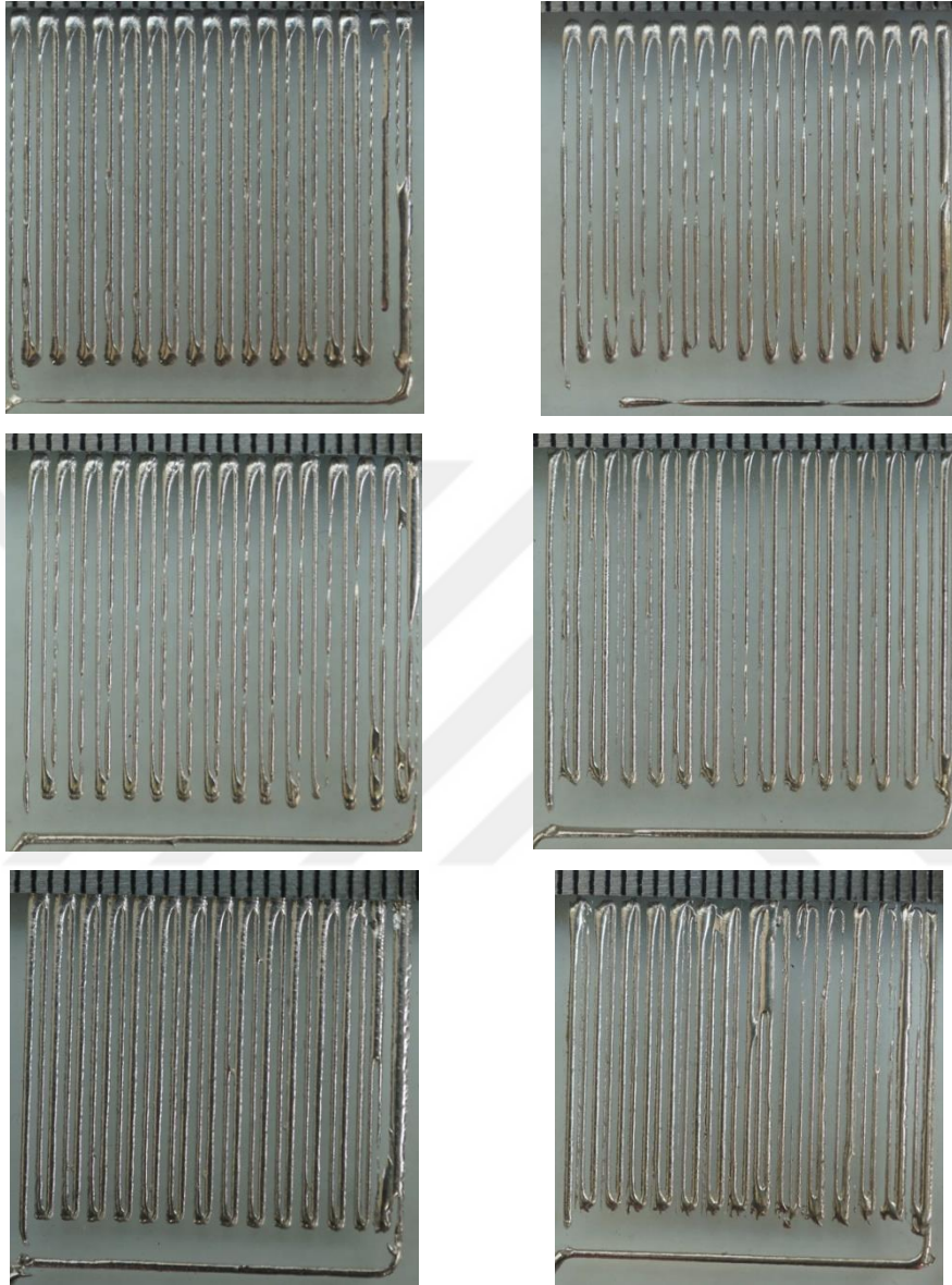
Figure 4.27. Infill samples printed using EM of 1, PS of 100 mm/min, LT of 0.2, PT of 75°C, ET of 160 °C
