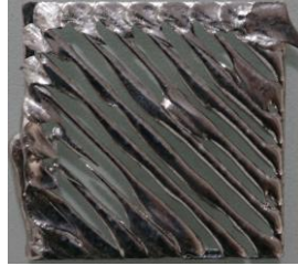
Figure 4.36. Square sample printed at printing speed of 100 mm/min, extrusion multiplier of 4, the layer thickness of 0,2 mm, platform temp of 75 °C, extrusion temperature 200 °C, and %50 infill
