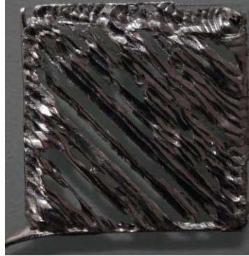
Figure 4.42. The solid square sample was 3D printed at an extrusion temperature of 180 °C, platform temperature of 75 °C, the printing speed of 100 mm/min, extrusion multiplier of 1, extrusion width of 0.3 mm, and 100% infill
