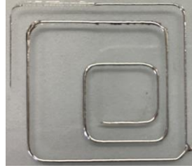
Figure 4.16. Close-up of a printed wireframe with a printing speed of 150 mm/min at 185 °C
