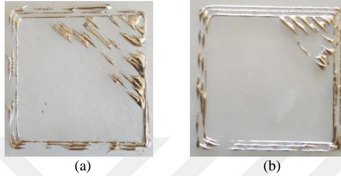
Figure 4.8. a) The square sample printed in ET of 143 °C, PS of 200 mm/min, EM of 1.15, LT of 0.2 mm using a 1.02 mm diameter brass nozzle, b) Square sample printed in EM of 1.15 and printing gap of 0.15 mm
