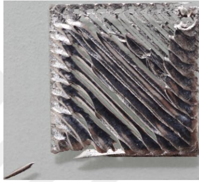
Figure 4.39. Obtained results for the solid square sample using extrusion temperature of 200 °C and table temperature of 75 °C with a printing speed of 100 mm/min, extrusion multiplier 1, and % 100 infill rate, respectively
