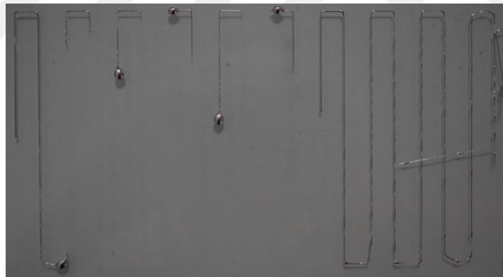
Figure 4.29. Printed maze geometry at an extrusion temperature of 140 °C
