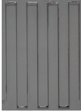
Figure 4.34. Sample printed at printing speed: 100 mm/min, extrusion multiplier: 1, layer thickness: 0,2 mm, table temp: 75 °C and extrusion temperature 200 °C
