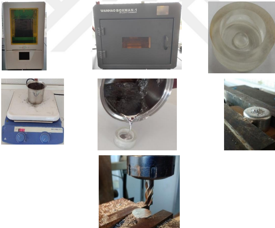
Figure 3.6. Applied casting process for the female mold production
