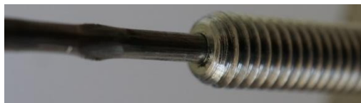
Figure 4.13. Deformed Bi58Sn42 filament due to the pushing and retraction movements during the printing process
